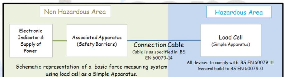
Simple Apparatus must be used with a safety barrier and installed in accordance with the following standards; BS EN 60079-25 Explosive atmospheres. Intrinsically safe electrical systems and the code of practice BS EN 60079-14 Explosive atmospheres. Electrical installation design, selection and erection.
