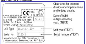
Our product label shown here, displays markings to indicate this. When these load cells are used as intrinsically safe load cells, that is, relying on ia protection concept then the energy supplied to these load cells **must** be limited. This energy limitation is achieved by the use of safety barriers which are special products we do not manufacture. Below is a brief explanation of the two types of safety barriers generally used in weighing applications with some key points about them,
